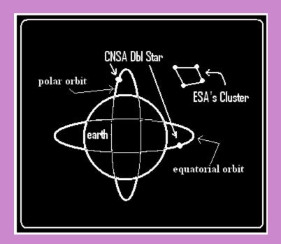
Double Star is a pair of satellites, one in an equatorial orbit and the other in a polar orbit, launched and operated by the China National Space Administration in collaboration with the ESA. Launched soon after Cluster, Double Star supplements the data collected and the two systems enable simultaneous data of the changing magnetic fields and ion population in different regions of the magnetosphere.
